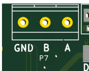
Illustration 3: Detailed View of Modbus Terminal
