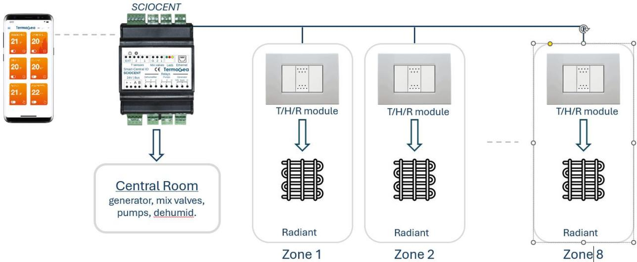
Even with this type of installation, both temperature and humidity are controlled in each area, thanks to the humidity sensor on the T/H/R module and the outputs for the dehumidifier of the SCIOCENT control unit.
