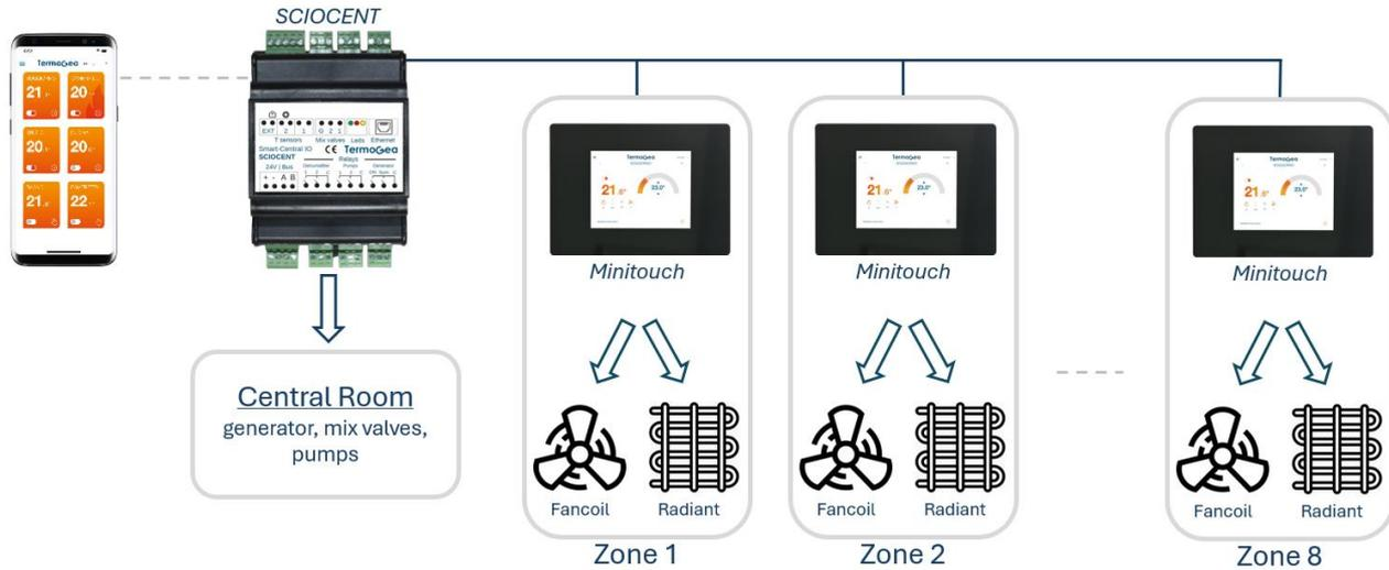
The circulation pump and the mix valve are activated by the thermostat function allowing the passage of the fluid in the radiant system. In Summer the de-humidistat function activates the dehumidifier and a second circulation pump dedicated to it. It is possible to control up to 8 zones independently.
