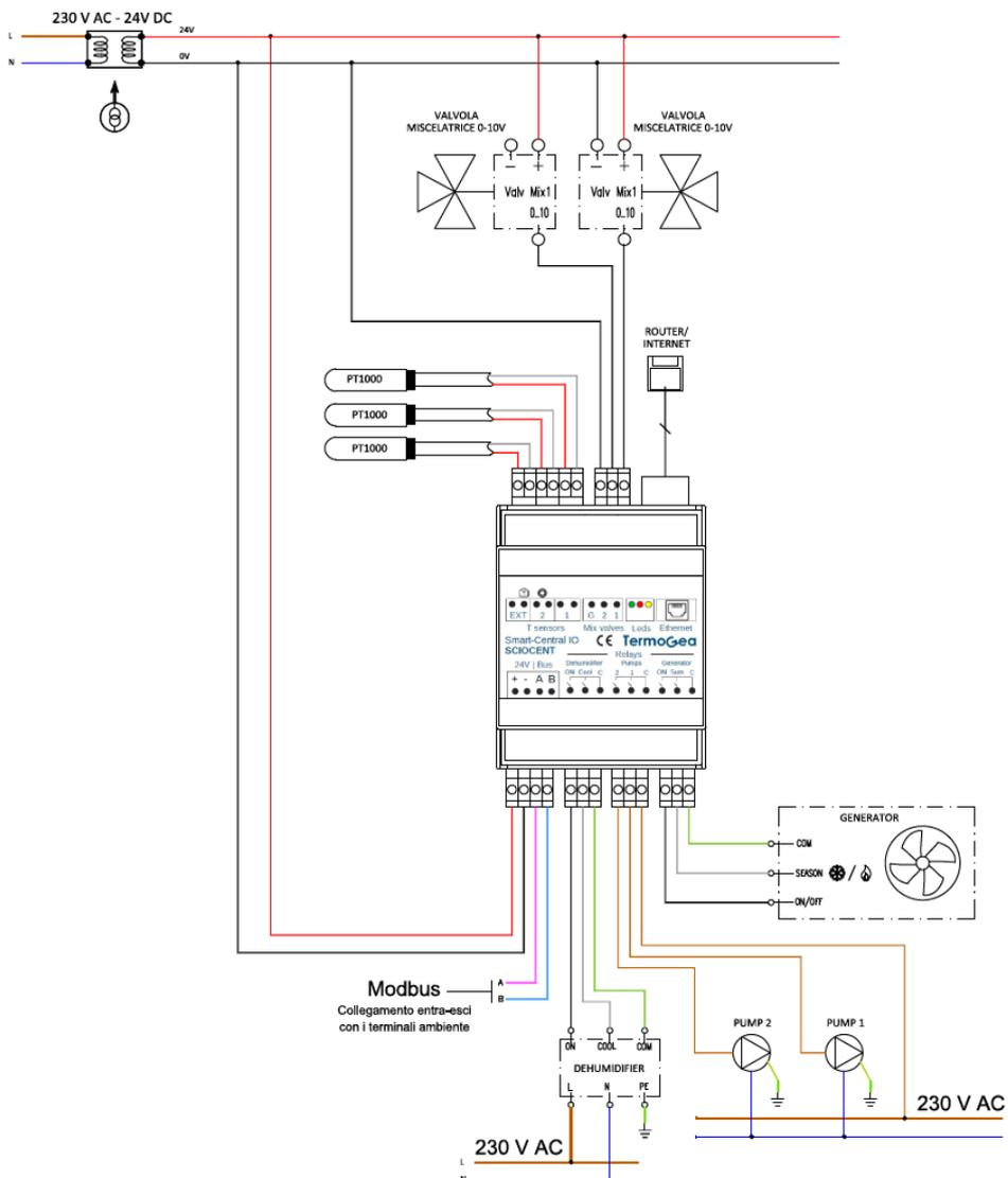
The "ROOM" or "MINITOUCH" thermostats or the "SND-THRT" probe-relay modules are connected to the MODBUS cable in the diagram.
