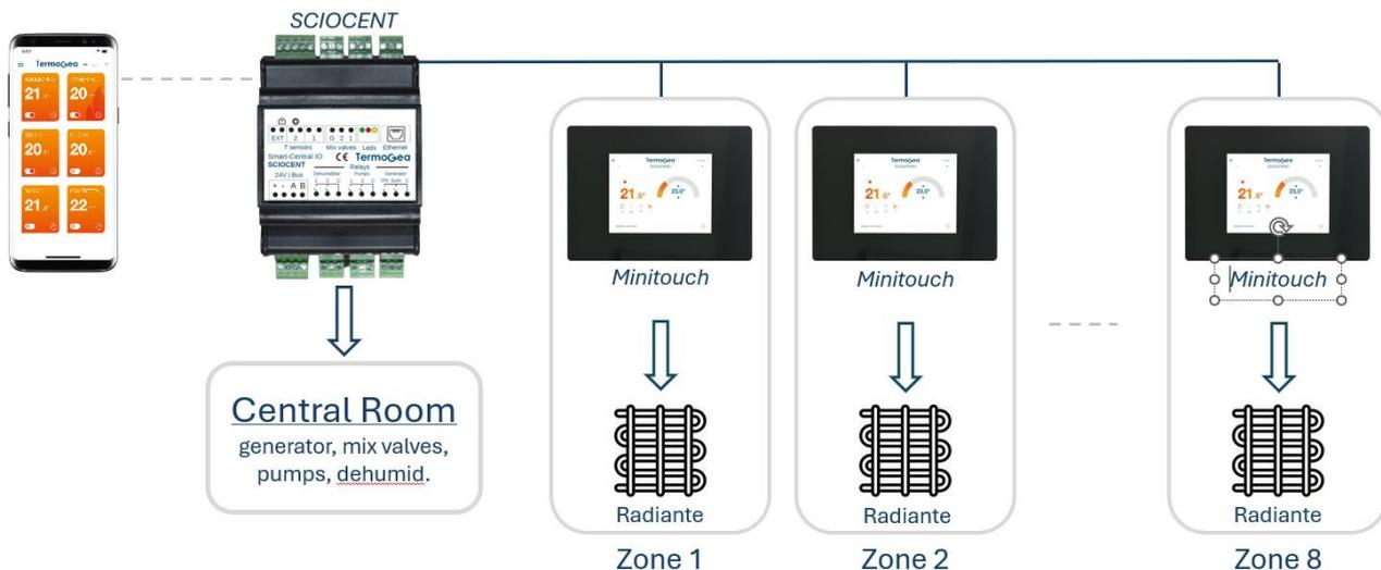
Even with this type of installation, both temperature and humidity are controlled in each area, thanks to the humidity sensor on the MINITOUCH and the outputs for the dehumidifier of the SCIOCENT control unit.
